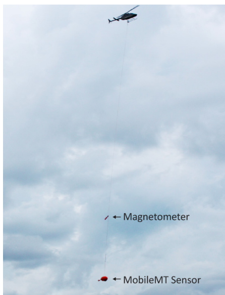
Figure 1: MobileMT bird towed by helicopter
