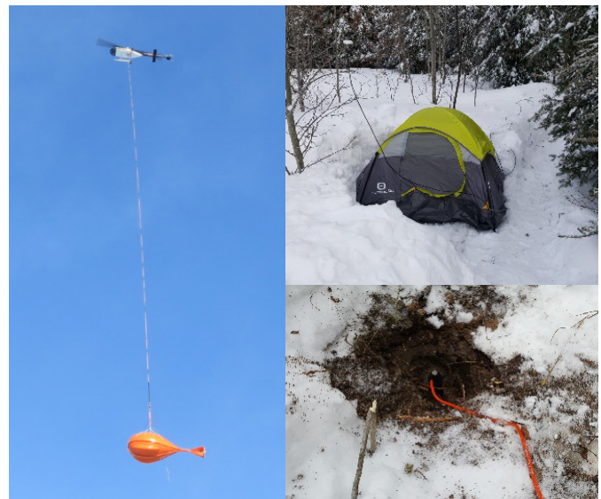
Figure 1: MobileMT bird towed by a helicopter (left), electric base station installation (top right), one of eight ground electrode installations (bottom right)
