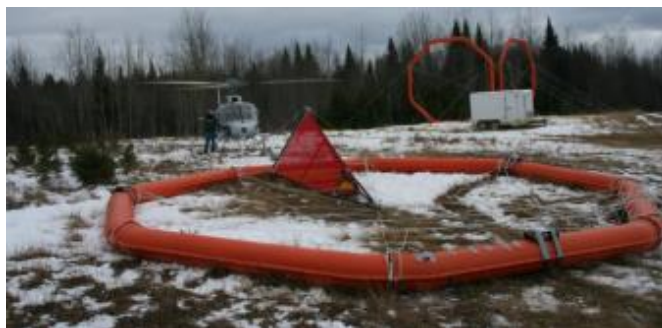
Figure 3: ZTEM z-axis receiver and ground-based prototype reference coils from field tests in northern Ontario, Canada in 2006 (after Lo and Kuzmin, 2008).
