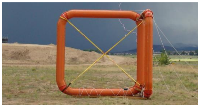
Figure 5: New (foreground) and old (background) ZTEM base station sensors, during field trials in Nevada USA in 2011(after Legault, 2012)
