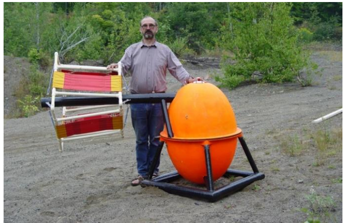
Figure 2: Geotech's airborne AFMAG system in field trials in Sudbury, Ontario with the principal designer, Dr. Petr Kuzmin. (after Lo and Kuzmin, 2004).
