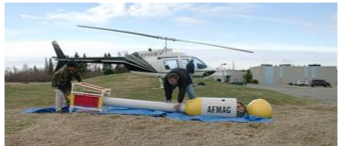
Figure 1: Towed-bird AFMAG prototype, 2001, (Kuzmin et al., 2005)
