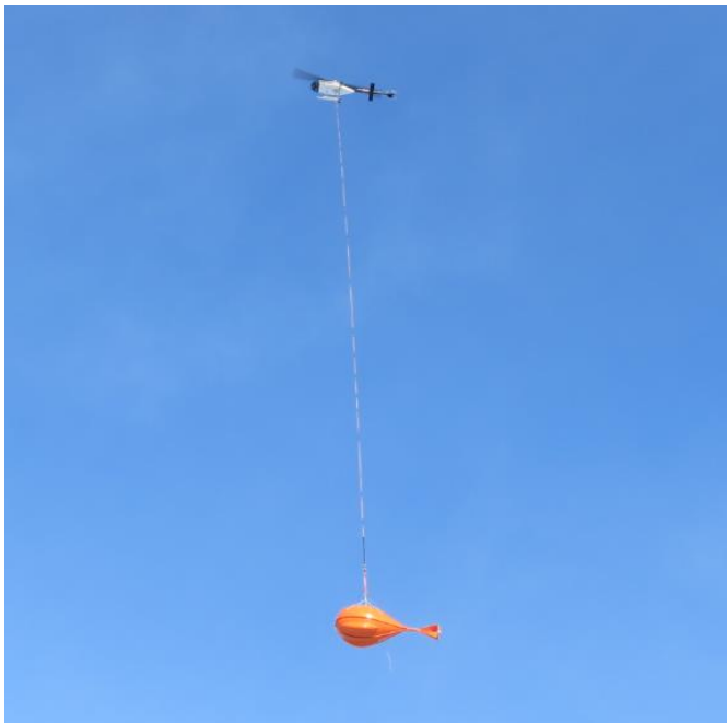
Figure 7: Helicopter MMT system in Cochrane, Ontario.
