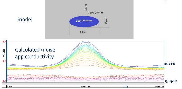
Rho y, RMS: 0.9581 invporph04-02fileroot.11.resistivity, Folder: case1
