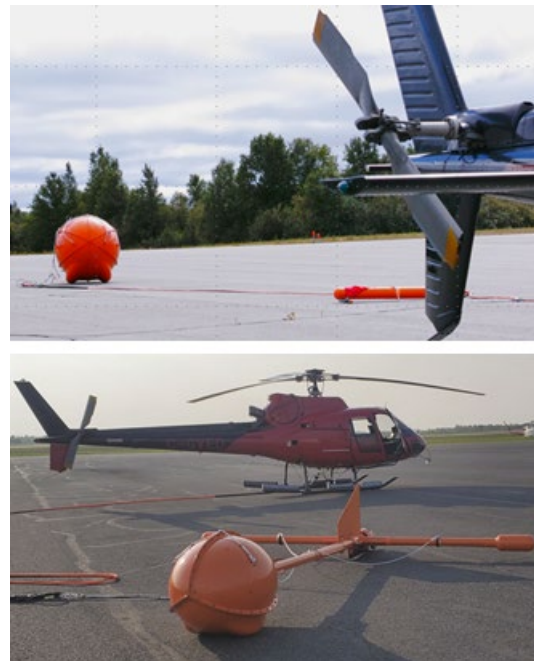
Figure 1. Airborne component of original MobileMT (top), and modified MobileMTm (bottom) systems.
