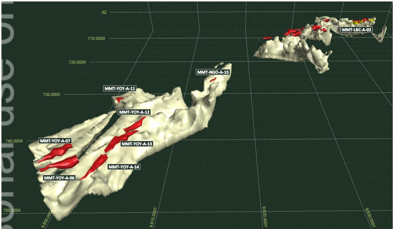
Figure 4: Location of the MobileMT targets along the Ngongo-Yoyo Trend (view looking west). Light green isoshells are 3D inversions of the MobileMT magnetic data. Red isoshells are interpreted MobileMT targets. The LMT trend with MobileMT targets is captured in the top right of the diagram for perspective - yellow isoshells are NSAMT targets from 2022 (refer to Company Announcement 14th November 2022). Target morphologies, strike length and depths have been considered during the interpretative phase. These targets remain untested by drilling programs - March 2023.
